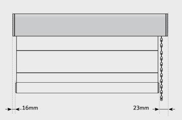
All component parts and fabric are enclose within a rounded resulting in a compact, robust system with a streamlined appearance. Fast, multiple installations can be achieved using top fix or face fix brackets that can be fitted along the whole length of the cassette. The snap fix fascia can be white or graphite or with a matching fabric profile.
