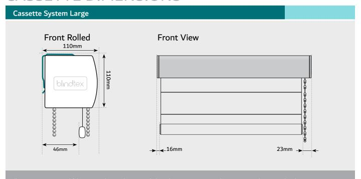
All component parts and fabric are enclose within a rounded resulting in a compact, robust system with a streamlined appearance. Fast, multiple installations can be achieved using top fix or face fix brackets that can be fitted along the whole length of the cassette. The snap fix fascia can be white or graphite or with a matching fabric profile.
