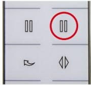
D) Then Press the Sync Button on the bottom right of the motor for 3 seconds until hearing beep sound
