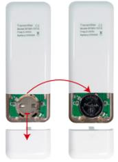
B) There are 2 small buttons to each side of the battery. The left side is the C button and the right side is the L button
