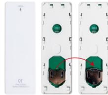
B) Select the channel you want to program with the bottom arrows. Channel 1 is on the left and channel 5 is on the right
